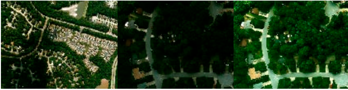
◀ Figure 3, UltraCamXp, 7 cm GSD: (left) whole scene, with dark area left caused by cloud shadows; (middle) pinpoint on dark area; (right) dark area after stretching grey values.
