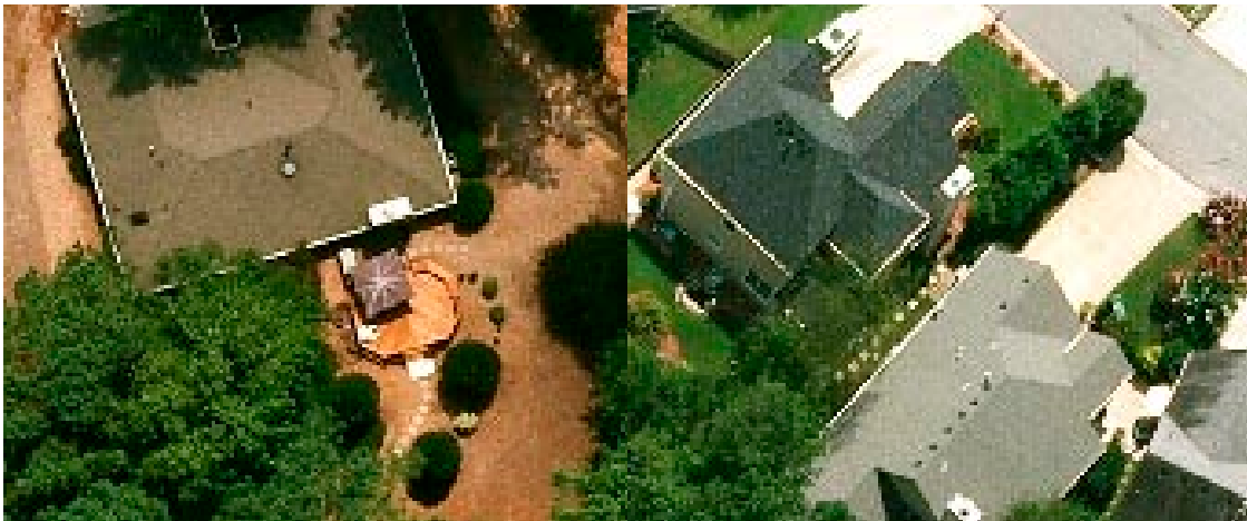
◀ Figure 5, Image sharpness across UltraCamXp image, 7cm GSD; pinpoints at centre of image (left) and corner (right).
