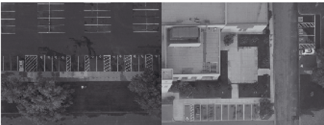
◀ Figure 6, Image sharpness across UltraCamL image, 10cm GSD; pinpoints at centre of image (left) and corner (right).
