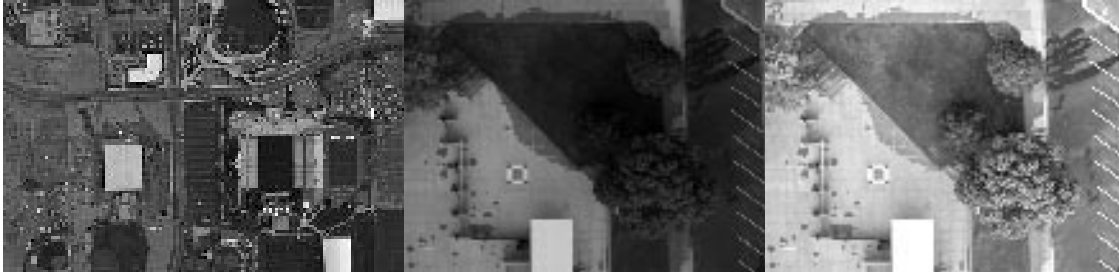
◀ Figure 4, UltraCamL 10cm GSD: (left) whole scene, with dark area left caused by cloud shadows; (middle) pinpoint on dark area; (right) dark area after stretching grey values.
